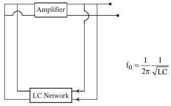
Part of output energy is sent back in phase to input circuit. This is also called positive feed back.
